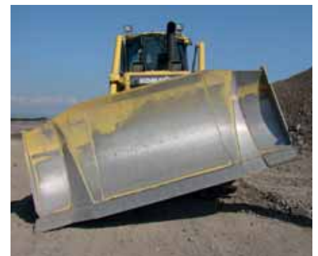
Hydraulically adjustable tilt: 870 mm
