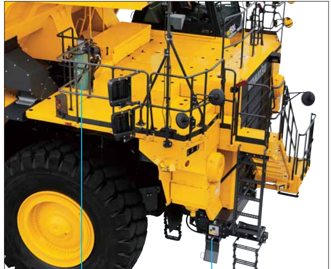
Grease pump and reservoir
